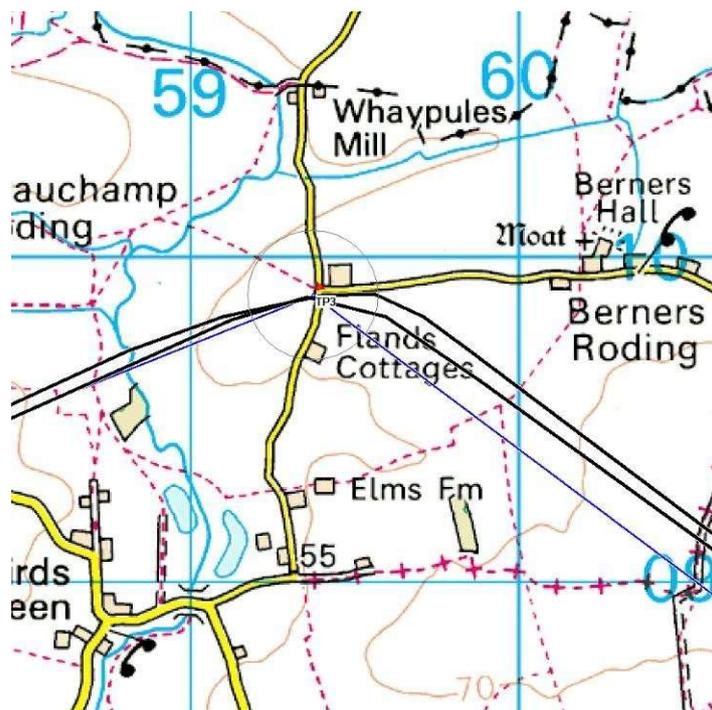
This looks like a perfect turn with the aircraft right above the turnpoint, however, the Rules state should the GPS trace pass inside the turnpoint by a distance of up to 8.5m then this will be classed as a "CUT" and a 5 second penalty will be applied to the aircrafts finish time.
